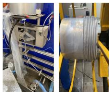
Wire casting machine (left) and coiled wire
