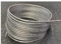
Cast wire batch (Al6063, Ø 9.5 mm, l 15 m)
