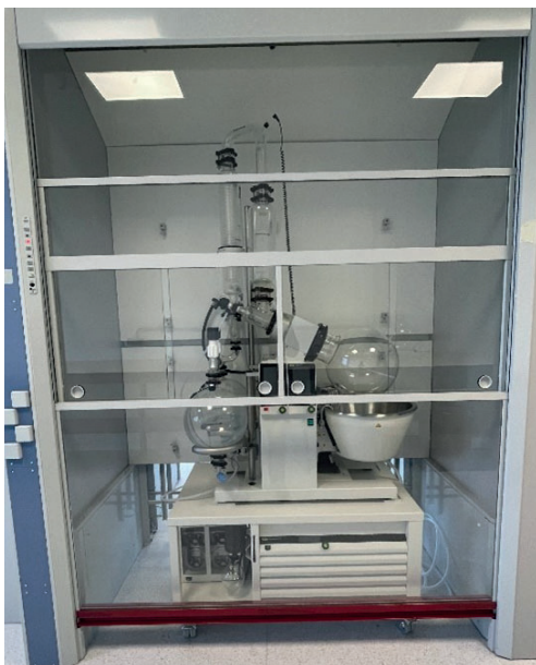
Figure 1: Rotary Evaporator Antwerp: a device used to purify and concentrate products in the lab
