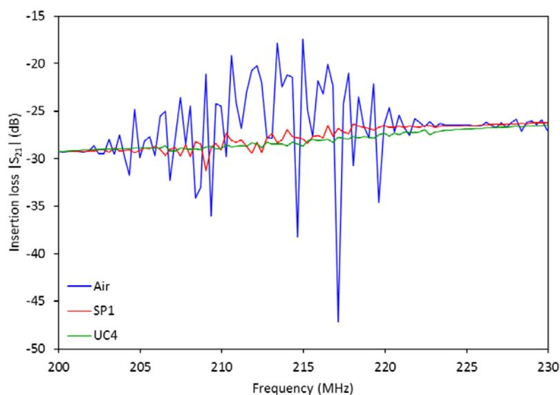
Figure 6 – Electrical response of SAW sensors exposed to air and to two samples containing different types of particles (SP1 and UC4). Despite the high attenuation, different shifts of the resonant frequency for each sample can be observed (SP1  $\approx$  5 MHz, UC4  $\approx$  2 MHz).
