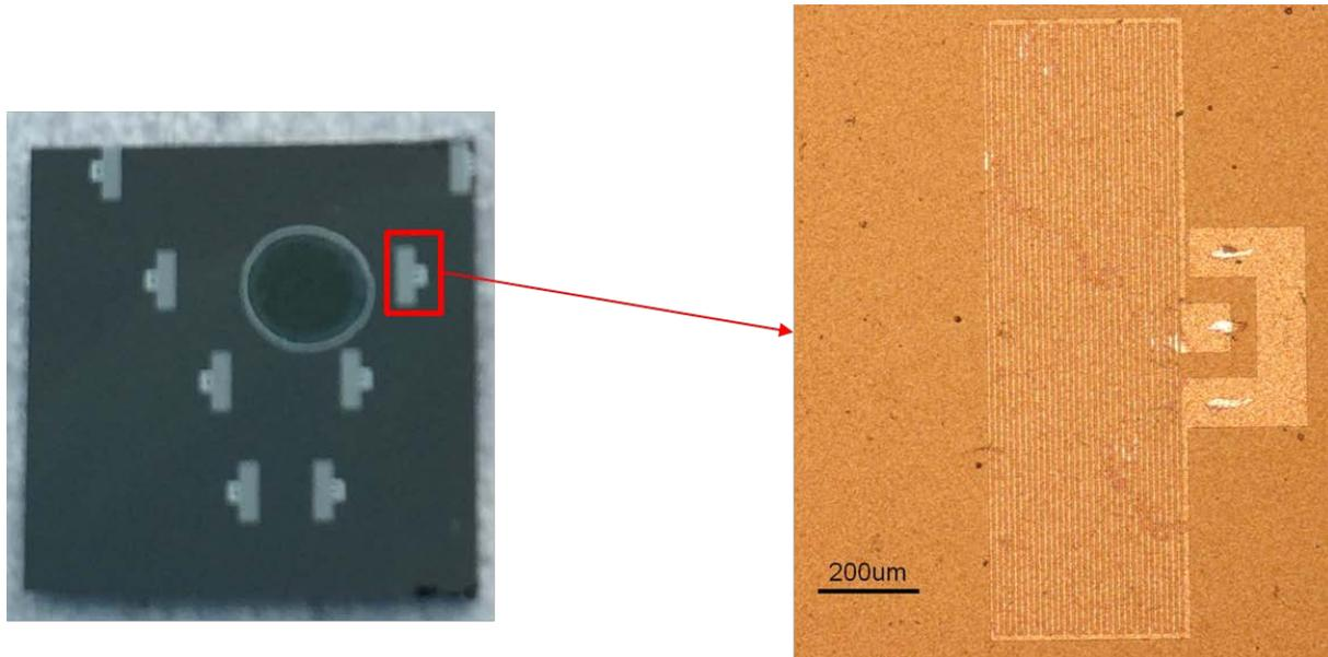
Figure 5 – Chip with four SAW delay line sensors and detail of the IDTs (pitch = 24  $\mu\text{m}$ , acoustic aperture 1.2 mm, number of finger pairs = 16) . The length of the sensing area varies in the different sensors (1.2 mm, 2.4 mm, 4.8 mm, 7.2 mm). A dried drop of emulsion used for the tests can be seen in the delay line.
