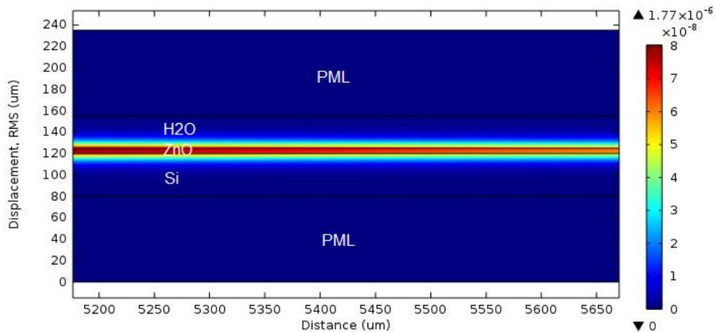
Figure 2 – RMS displacement map in a plain SAW device. The acoustic energy is concentrated in the piezoelectric layer, with exponentially decaying tails in the water and the substrate. The coloured displacement scale is in metres.
