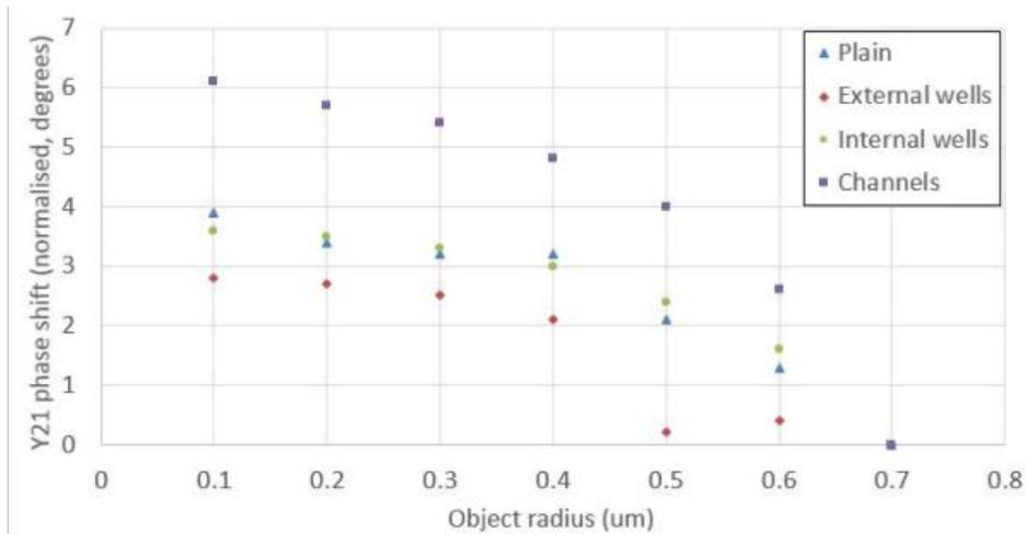
Figure 4 – Summary of results from 3D simulations for various surface texturing options. Phase shift was normalised to 0° for 700 nm object radius to facilitate sensitivity comparison.
