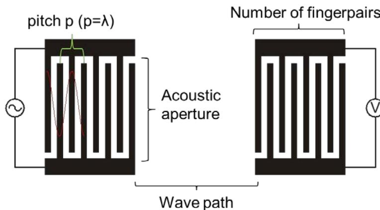
Figure 1 –Sketch of a delay line with the design parameters.
