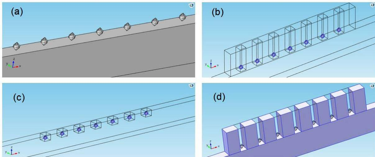
Figure 3 – Surface texturing options simulated with 3D FEM numerical methods: flat surface (a), external wells (b), internal wells (c), and channels (d). In all cases, surface particulates are included in the simulations.
