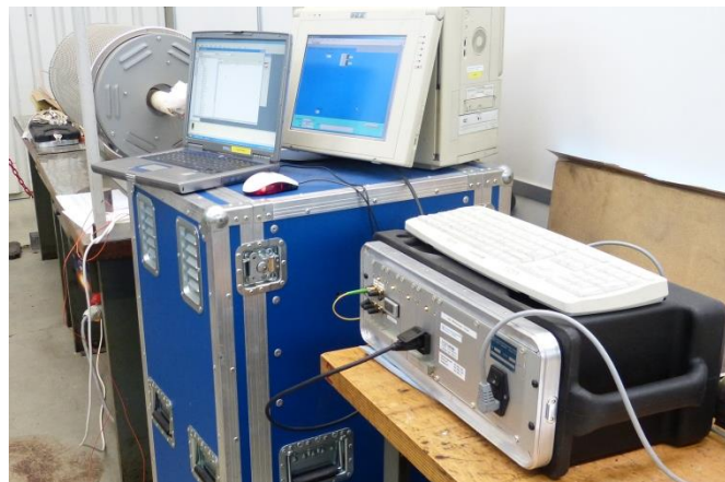
Figure 2: Experimental setup of heat resistance test with tube furnace (left), notebook for data evaluation (mid), and interrogator with applied fibre optical sensor (right)
