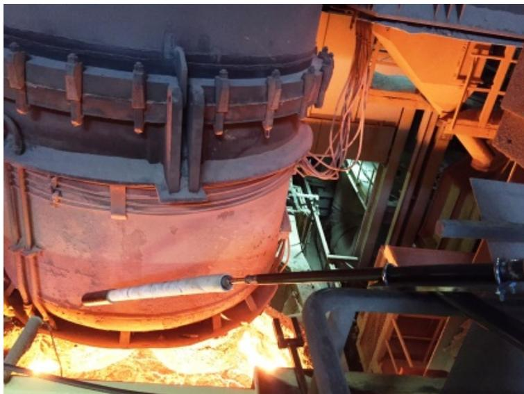
**Figure 2:** Photograph of the novel probe and the adapted hand lance for temperature measurements in front of the vacuum degassing plant
