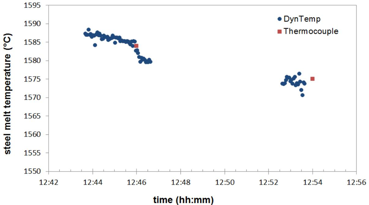
**Figure 5:** Detailed graph of the evolution of the liquid steel temperature during the start of vacuum degassing as measured by fibre optical and thermocouple measurements.
