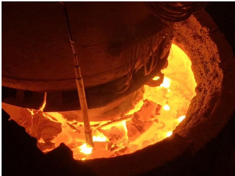
**Figure 3:** Photograph of the hand lance for long term temperature measurements in the ladle during vacuum degassing.
