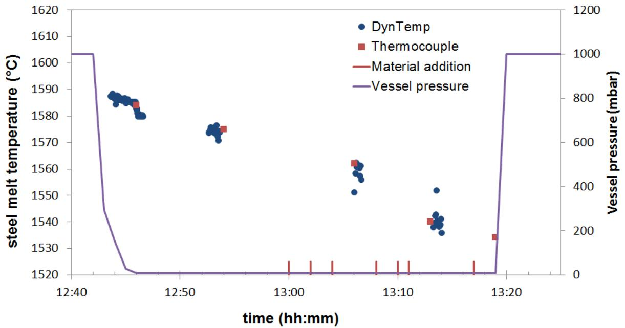
**Figure 4:** Graph of intermittent measurements of the liquid steel temperature evolution (left axis) together with other process data (right axis).
