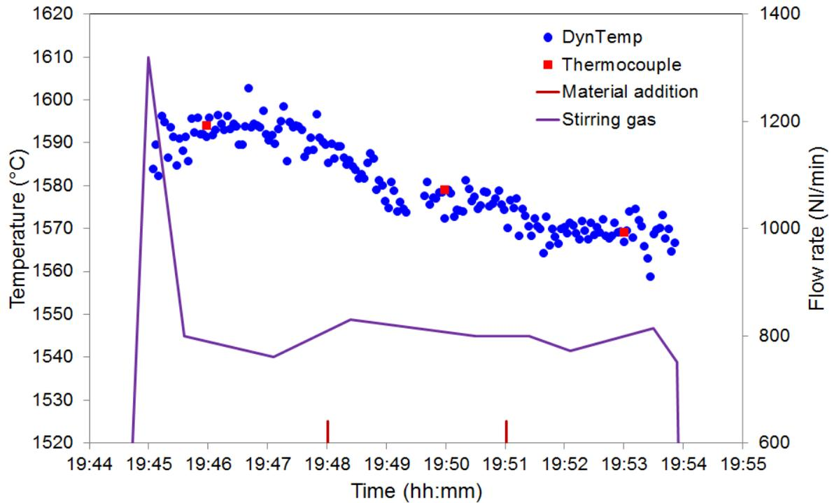
Figure 4: Liquid steel temperature evolution during gas stirring using an adapted stirring lance as measured by fibre optical and thermocouple measurements.
