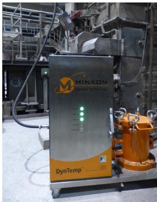
Figure 1: Photograph of the demonstrator for fibre optical temperature measurements installed at the Ar stirring stand of TKSE
