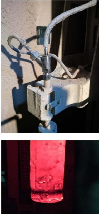
Figure 2: Photograph of a y-junction at the cold end of the stirring lance and the blowing nozzles at the hot end of the stirring lance
