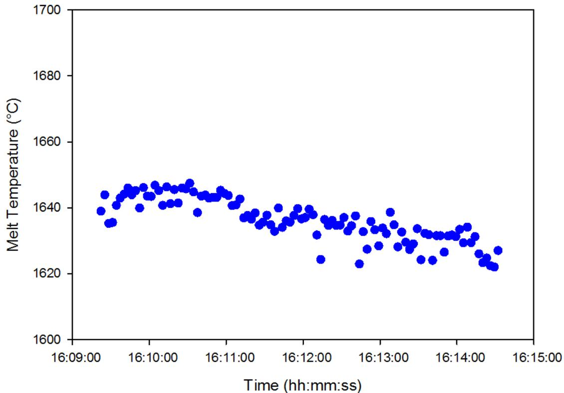
Figure 3: Liquid steel temperature evolution during gas stirring using the original stirring lance as measured by fibre optical system
