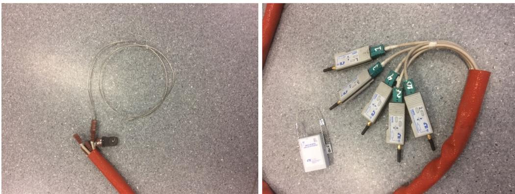
Figure 2 - Thermocouples for refractory measurements (left) and transmitters (right).
