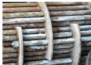
Figure 2. Fouling on a heat exchanger for a particular material might be poorly understood. Here plant data can be used to develop a data-driven model that captures this fouling behaviour.
