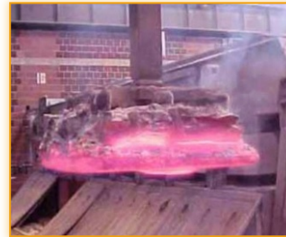
Anode flatness defect
