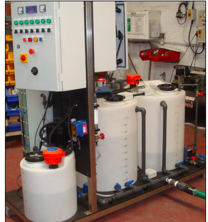
Gen II water unit is being lifetime tested
